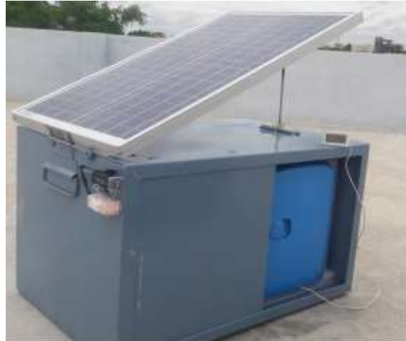
Fig 5. Construction of a portable solar refrigerator
