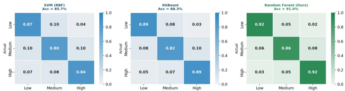
Figure 2: Normalised confusion matrices — SVM, XGBoost, and Random Forest (Test Set, n=707). Numbers indicate per-cell classification rate.
